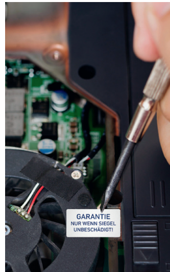
Figure 3: Heat-resistant guarantee seal based on ultra-destructible acrylate security labelstock
