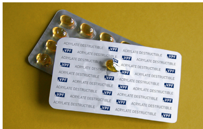
Figure 2: When blisterpacks are overlabelled, it must still be possible to press out the contents with ease.
