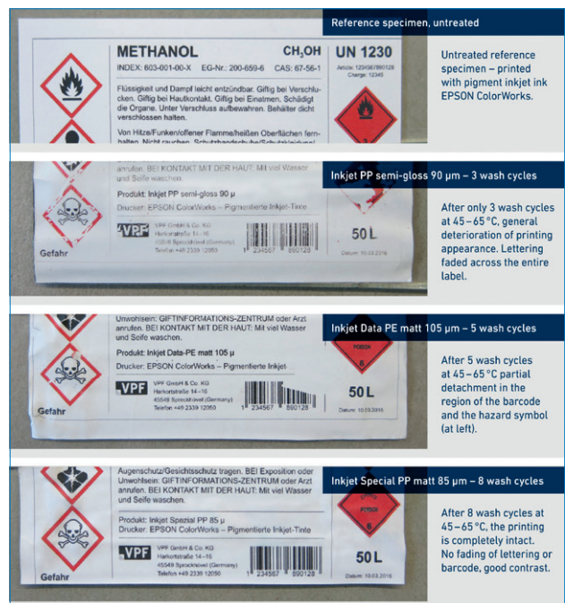
Figure 3: Resistance of different inkjet films compared to an untreated reference sample
