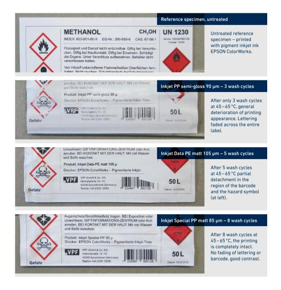
Resistance tests of the newly developed Inkjet Special PP white matt 85  $\mu$ m film after several washing cycles at 45 to 65 °C compared to conventional Inkjet PP and PE reference materials.
