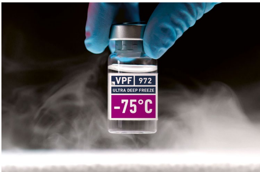
VPF 60659 PP white glossy with adhesive 972, 18\text{g}/\text{m}^2 after storage at -75^{\circ}\text{C} .
